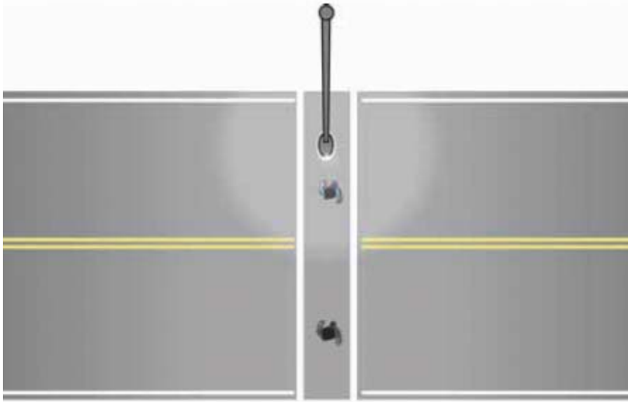
Fig 11. Traditional midblock crosswalk lighting layout
